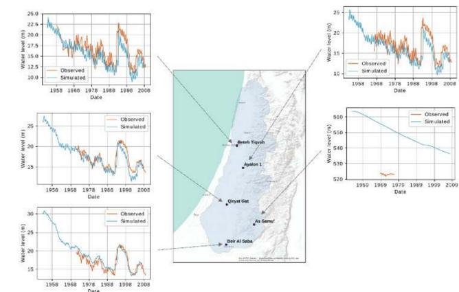
Figure 6: Computed vs. observed transient hydraulic heads
